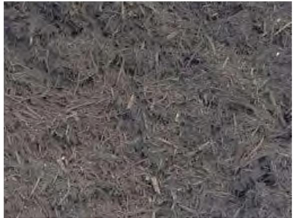
This BMP consists of applying a mixture of shredded wood mulch, bark, or compost to bare soil to reduce runoff, increase infiltration, and reduce erosion due to wind or rainfall impact. Wood mulch provides temporary or short-term soil stabilization. This material should be applied to exposed soil beneath the existing tree canopy along the eastern edge of the facility and adjacent to Arnold Road.
